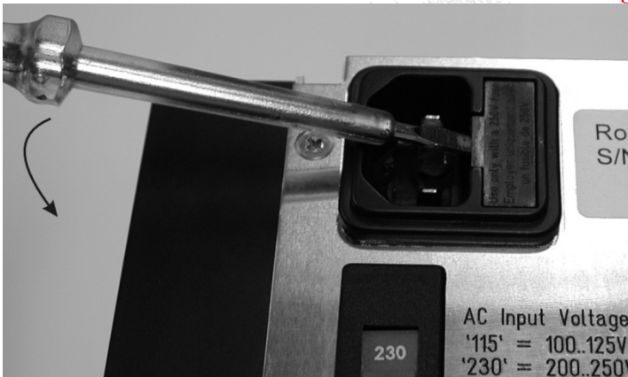
Figure 2.1: How to remove the input fuse
